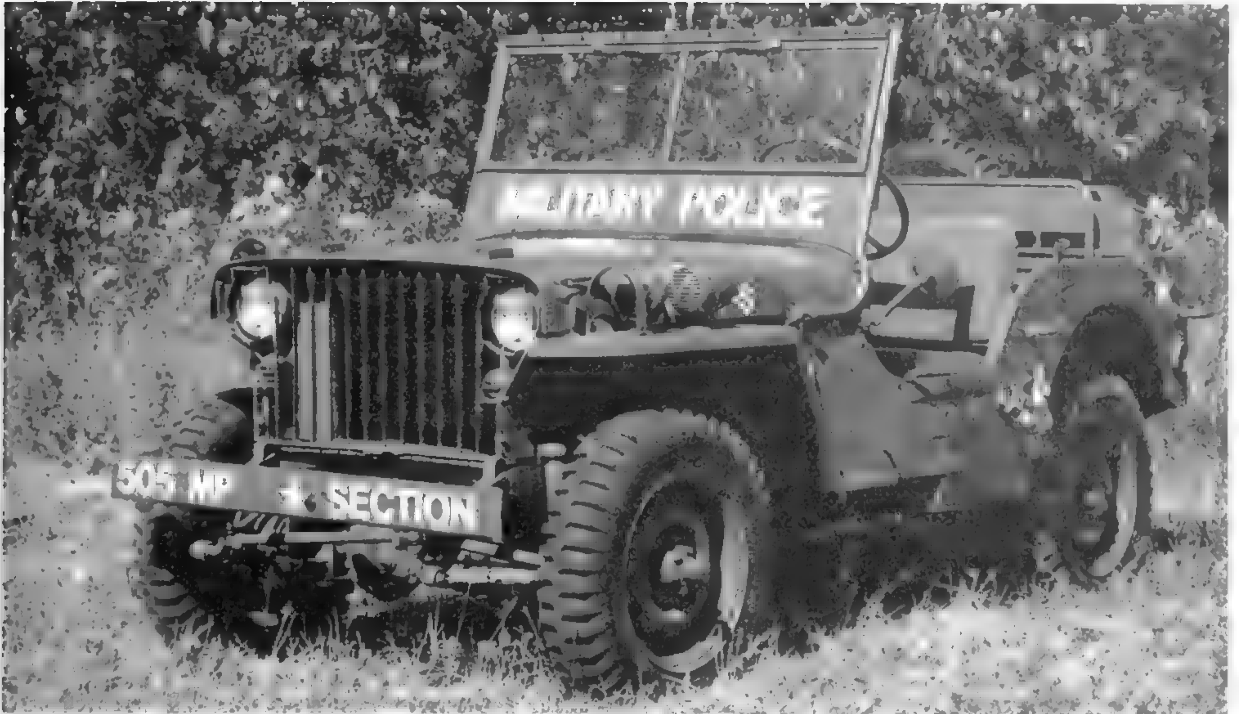
After extensive field testing of the MA, the design was improved and standardized as the MB. The first 25,808 of these featured what collectors refer to as a "slat grille." This was a welded assembly of heavy bar stock. (Photo courtesy of Reg Hodgson)
